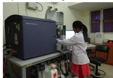
BD FACS Aria III cell sorter with a 5 laser (Near UV-375nm, Violet-405nm, Blue-488nm, Yellow—Green-561nm, Red-633nm) and 11 color setup has a throughput of 70,000 events per second and can do one-way, two-way, three-way, 4-way sorting and single cell sorting.
